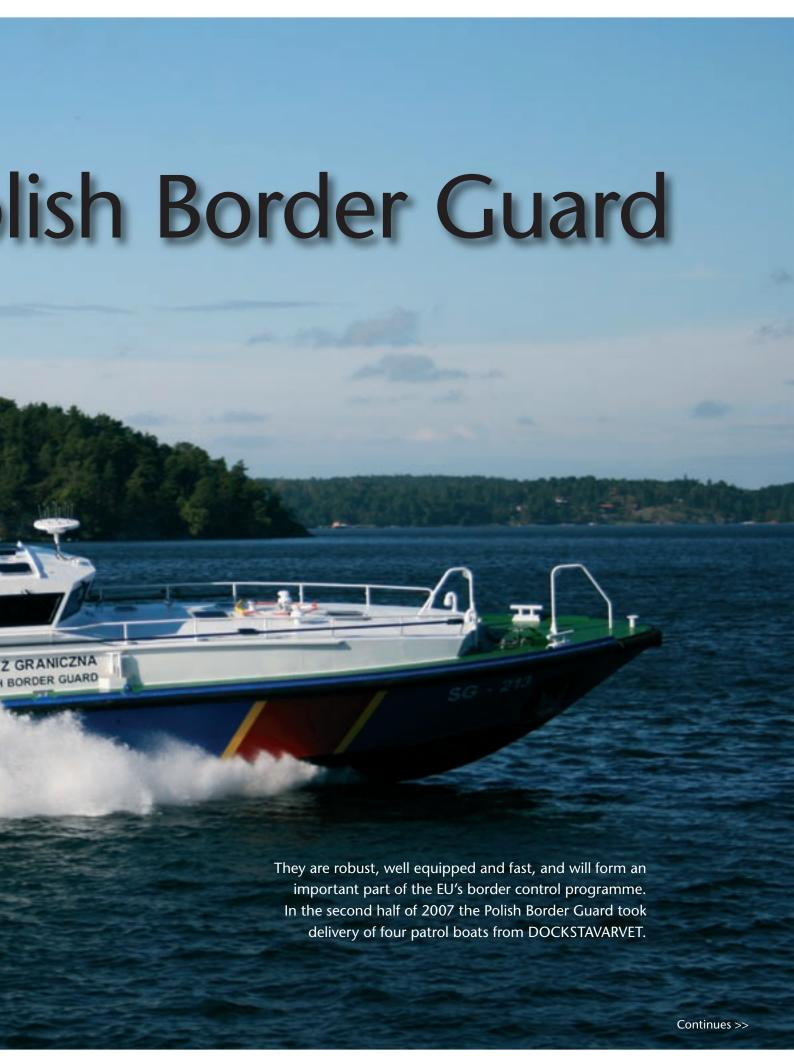
The almost mirror-like surface of the bay outside DOCKSTAVARVET, a 100 km north of Sundsvall, is cleft asunder by the V shaped aluminium hull, speeding along at over 40 knots. The hull's tried-and-tested 20 degree deadrise ensures a smooth ride and makes the boat easy to manoeuvre, adding to its excellent sea-keeping qualities. After a few minutes Project Manager Per Öberg slows down and steers back towards the wharf.
