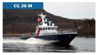
Length over all20.190 mBeam4.65 mDisplacement35 tonsEngine power2 x 374.5 kWSpeed20 knots
