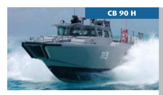
Length over all14.90 mBeam3.85 mDisplacement18 tonsEngine power2 x 600 kWSpeed45 knots
