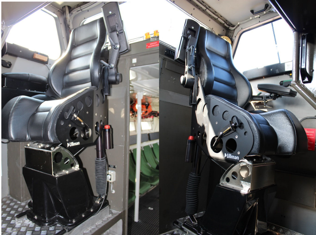
The Wheelhouse on Enforcer III is fitted with two Ullman Atlantic Seats for the Helmsman and Navigator.
